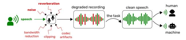
Speech enhancement consists of improving the quality and intelligibility of speech in a degraded recording, for instance due to interfering sound sources and reverberation (Vincent et al., 2018). The task is to estimate a clean speech signal from the degraded recording, as illustrated above. Speech enhancement finds applications in various speech technologies for human and machine listening (hearing aids, assistive listening devices, vocal assistants, etc.)
